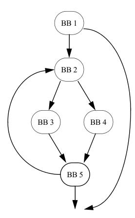
16. Assume that an one-bit (history bit) state machine (see above) is used as the prediction algorithm for predicting the execution of the two branches in this loop. Indicate the predicted and actual branch directions of the b1 and b2 branch instructions for each iteration of this loop. Assume initial state of 0, i.e., NT, for the predictor.
